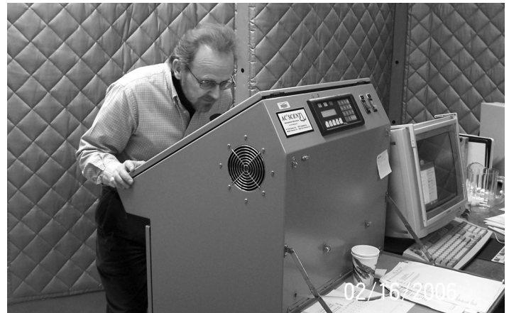
Figure 4. St. Croix Sensory Ac'Scent Olfactometer is portable and costs about $50,000. Labs charge up to $1,000 per sample.
