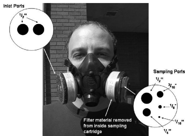
Figure 3. Constructing a facial mask field olfactometer requires respirators and cartridges that can be found at most paint or fertilizer supply companies.
