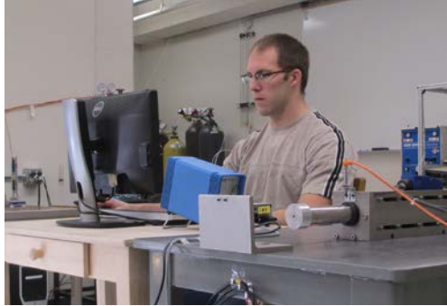
Samuel Van Horn works on a novel experimental apparatus that simulates the single compression stroke of a combustion engine using experimental fuels.
