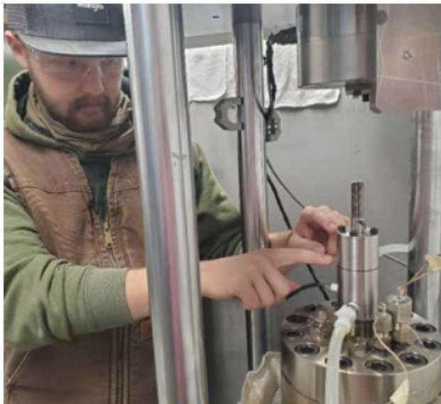
Cody Gibson's new cooling jacket implements a fail-safe design, which is critical for the extreme environmental conditions.
