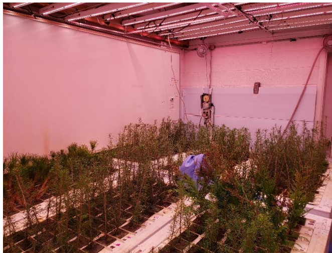
Conifer seedlings in the root growth potential aeroponic mist chambers in the CFNSR Seedling Quality Lab.
