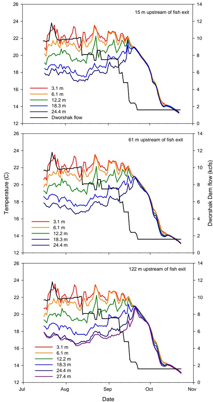
Figure 22. Lower Granite forebay temperature logger data collected upstream of the fish ladder exit (top panel 15 m upstream), middle panel (61 m upstream) and bottom panel (122 m upstream) and Dworshak Dam flow in 2013.
