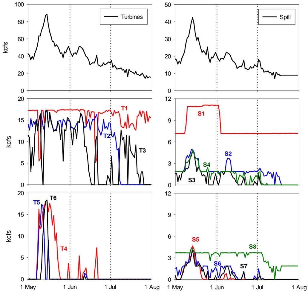
Figure 13. Mean daily turbine (T1-T6) and spillbay (S1-S8) discharge data (kcfs) from Little Goose Dam during the spring–summer Chinook salmon run in 2013. Note different y-axis scales.
