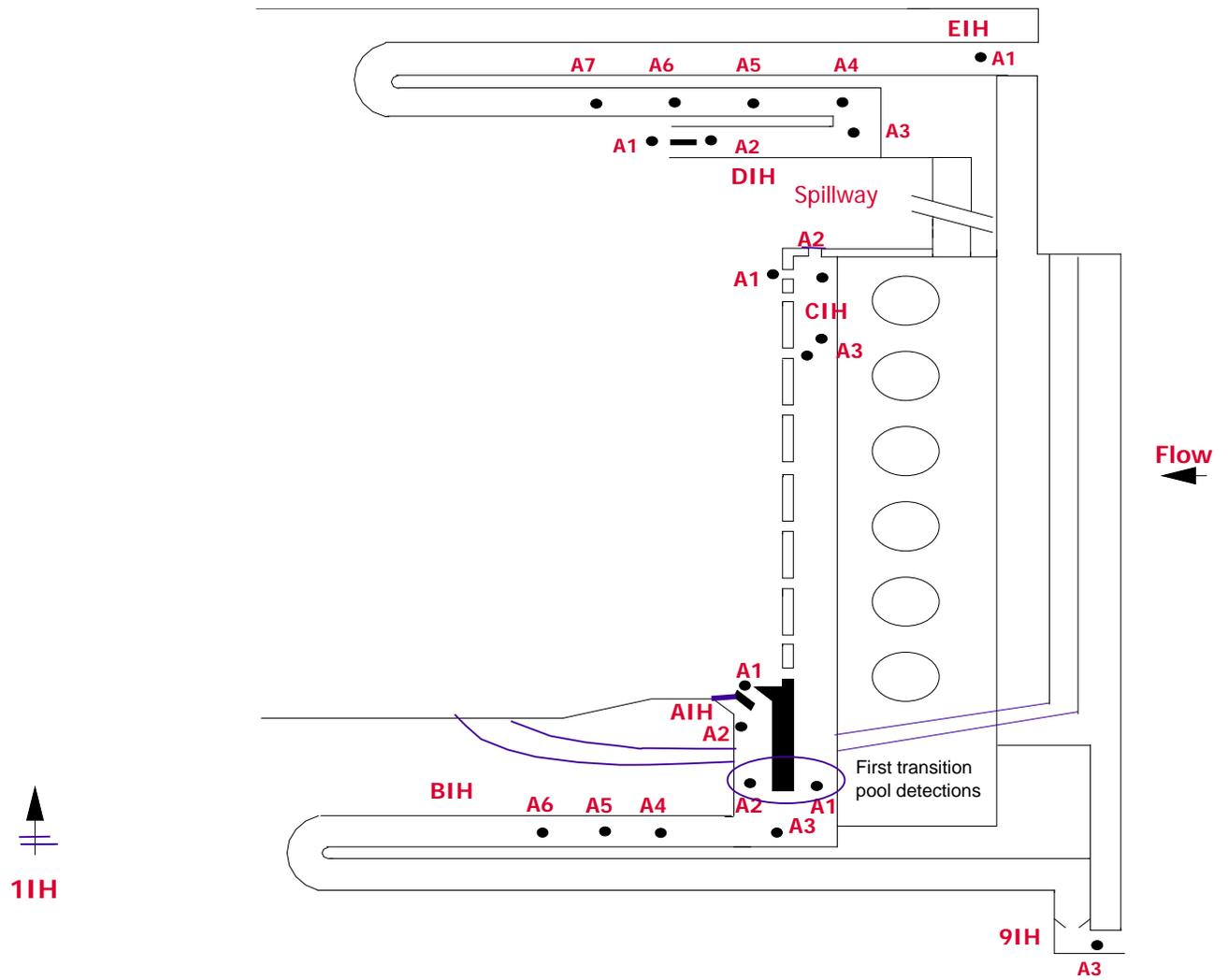
Figure 4. Locations that water temperature loggers and radiotelemetry antennas were deployed inside the Ice Harbor Dam fishway in 2013. (Not to scale.)
