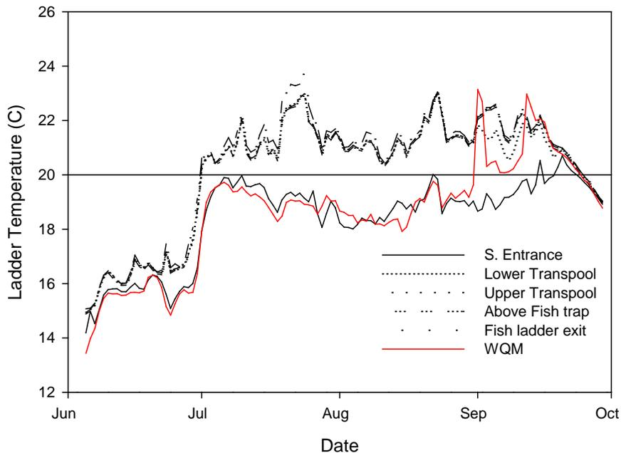
Figure 20. Daily average water temperatures at the five monitored locations in the Lower Granite Dam fish ladder in 2013 (black lines) and at the water quality monitoring site (red line).
